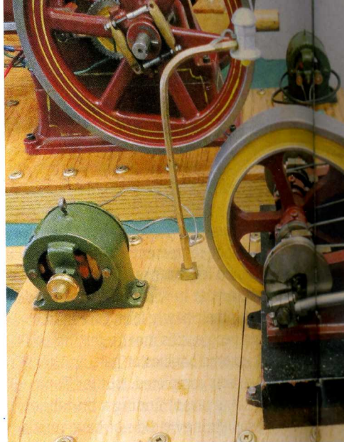
Another single-flywheel twin has been set up to run a small dynamo.
